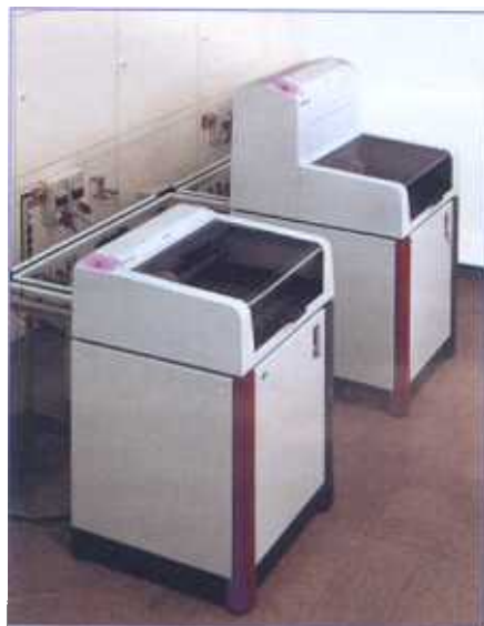
Figure 1. X-ray spectrometer S4 EXPLORER and diffractometer D4 ENDEAVOR integrated into an automated laboratory.
