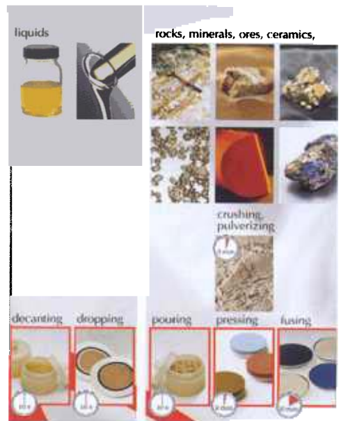
Figure 4. Simple and fast sample preparation for element analysis by XRF
