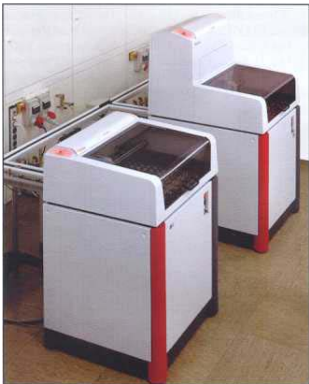
Figure 4. An X-ray spectrometer S4 Online used for chemical analysis and a diffractometer D4 Online used for quantitative phase analysis.
