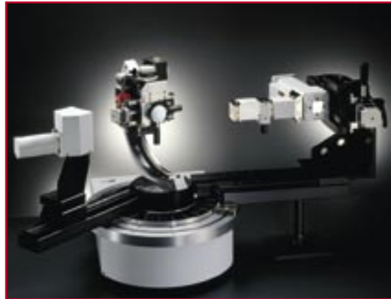
Fig. 3: For all other applications the line focus beam is perpendicular to the scattering plane.
