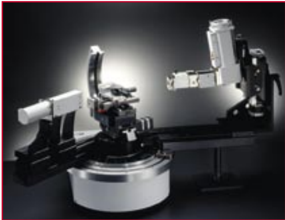
Fig. 2: In the IP-GID configuration the line focus X-ray beam is oriented parallel to the scattering plane.
