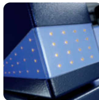
X-ray warning lights
