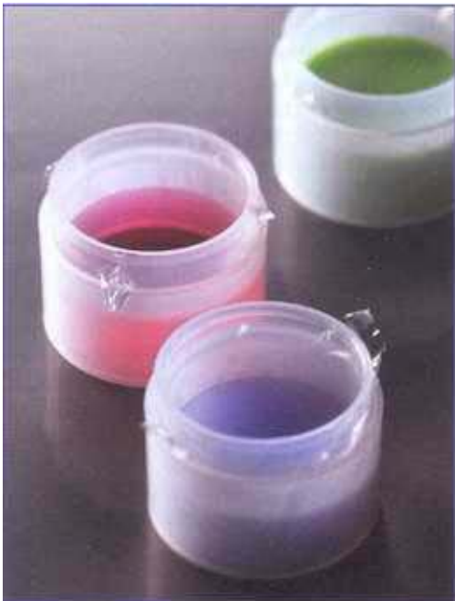
Figure 1. Disposable liquid cups for XRF analysis of liquid petrochemical products.
