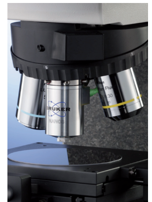
Close up of the NEOS turret: AFM scanning head is ready to engage for the measurement
