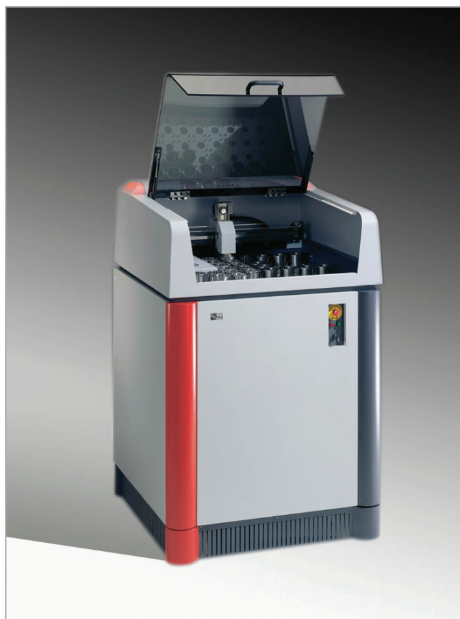
Figure 1 - Bruker AXS S4 PIONEER wavelength dispersive X-ray spectrometer.
