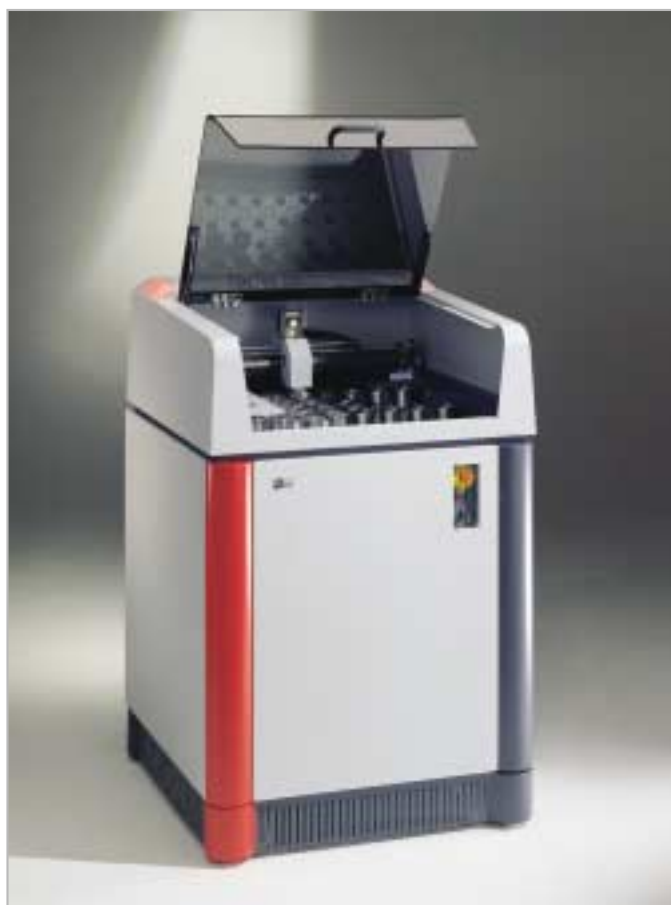
Figure 1 - Bruker AXS S4 EXPLORER wavelength dispersive X-ray spectrometer.
