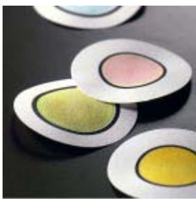
Figure 2: Filter paper with hydrofobe ring
