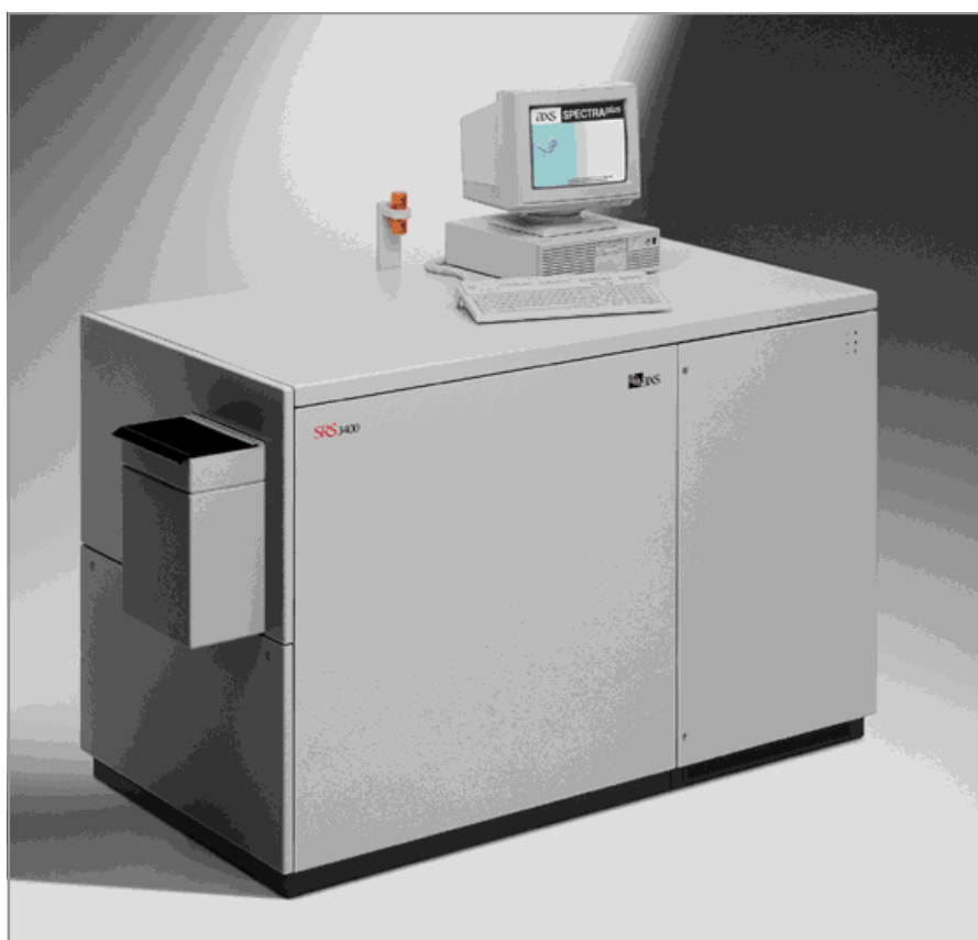
Fig. 1: Modern sequential X-ray spectrometer (SRS 3400)
