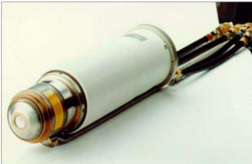
Fig. 2: Very close optical coupling of X-ray tube and an extremely thin beryllium window improve light element analysis (Siemens end-window X-ray tube)
