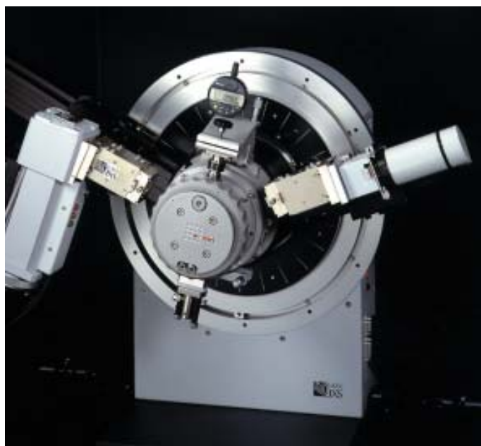
Fig. 1 Reflectometry chamber mounted on a D8 ADVANCE with twin Göbel Mirror TGM arrangement.
