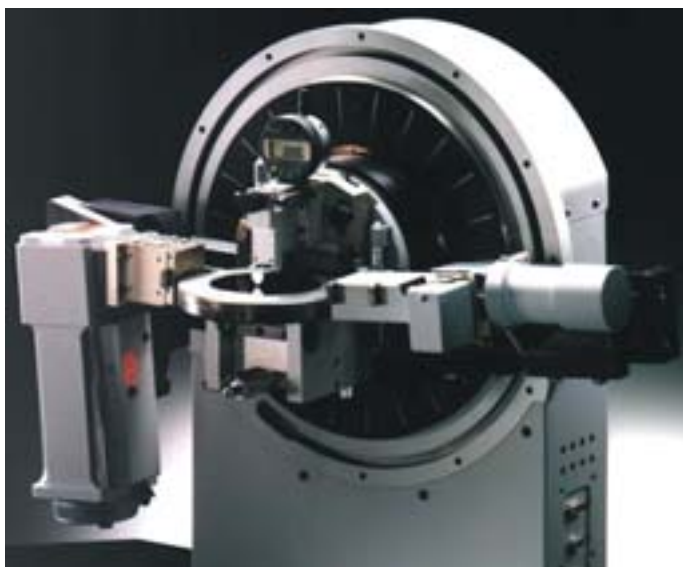
Fig. 2 - D8 ADVANCE goniometer with incident beam Göbel Mirror, reflectometry sample stage, fixed slit assembly with automated absorber and scintillation counter.
