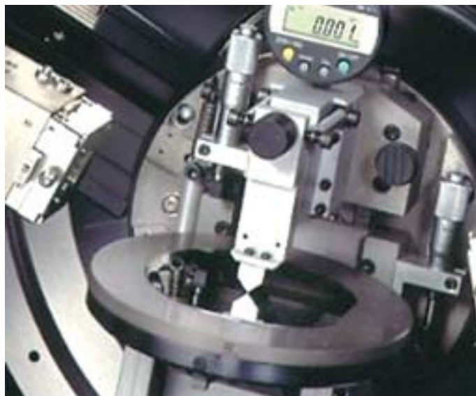
Fig. 3 – Reflectometry sample stage with Knife Edge Collimator. The dial indicates a distance of 1 \mu\text{m} between sample surface and knife edge.
