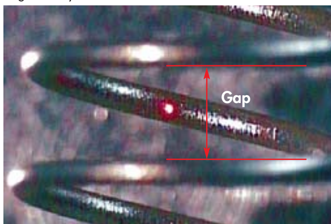
Figure 2: The video image showing a section of the spring. Both incident and diffracted beams can pass through the gap between the wires.
