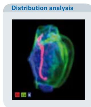
Fig. 2 Distribution of main constituents for 10 ms measurement time per pixel and approx. 5 min total measurement time
