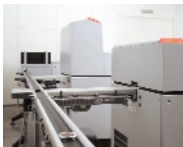
Figure 5: Laboratory automation concept with full integration of XRF and XRD analysis
