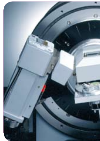
Set-up with energy dispersive SOL-XE detector
