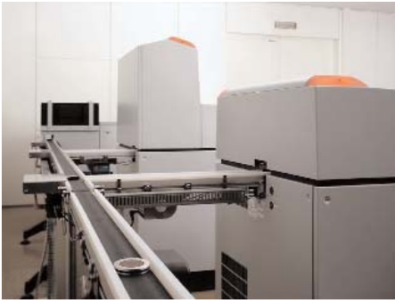
Figure 5. Easy integration of analytical X-ray instruments into process automation taking over, for example, process samples from a conveyor belt.
