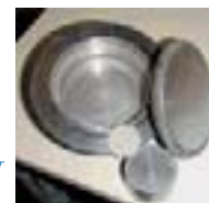
Fig. 4: Sample grinding with Vertrel XF results in a clean container with no contamination.
