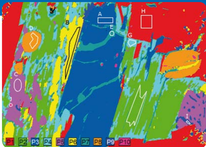
Phase analysis result of a granite sample. (Sample courtesy of the Berlin Museum of Natural History)
