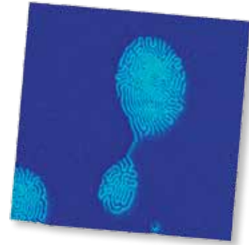
Polymer brush structures imaged on a MultiMode 8. Scan size 750 nm. (Sample courtesy of S. Sheiko, University of North Carolina, Chapel Hill)
