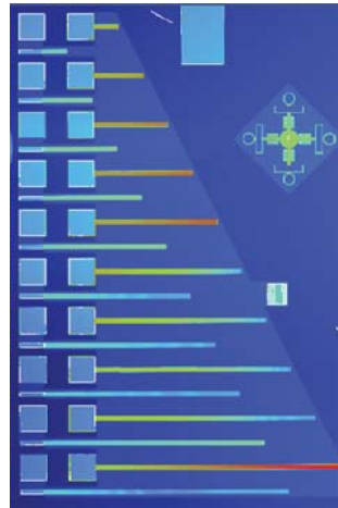
Figure 4. Topview perspective of a single (not stitched) optical profiler image, depicting twenty cantilever beams all at once. 1.4mm x 2.1mm area; 17 \mu m height range (color scale).
