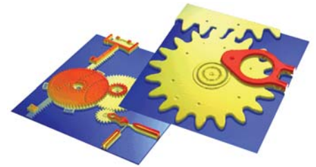
Figure 6. Foreground: a single high magnification (50X objective lens) optical profiler image with a lateral spatial sampling interval (pixel size) of 0.3 \mu m. The Veeco NT3300 and MEMS3500 optical profilers can stitch several such images into a mosaic, combining large field of view and high lateral resolution. Background: composite stitched together from 49 individual images (with some overlap at the boundaries); 580 \mu m x 640 \mu m area, 15 \mu m height range.
