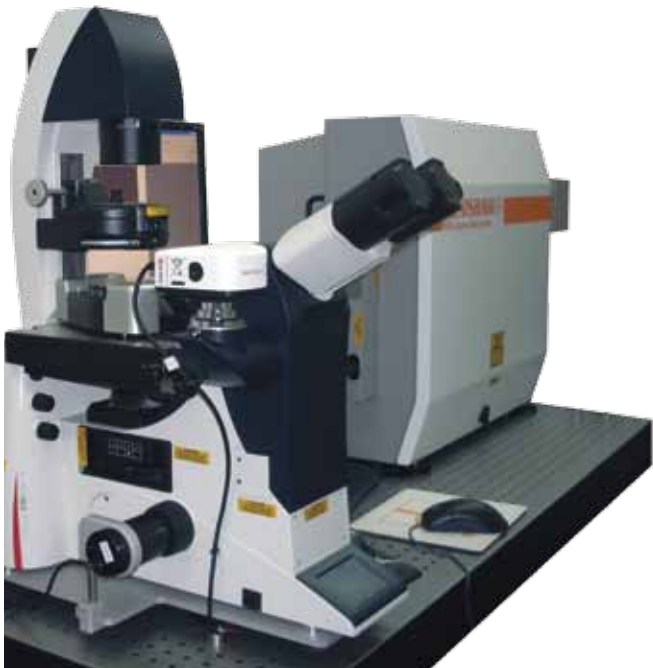
AFM-spectrometer integration example. This system leverages the unparalleled optical access of the BioScope to allow the most sensitive Raman detection. Courtesy of Aleksander Balter, Physics Department, UMK, Toruń, Poland.
