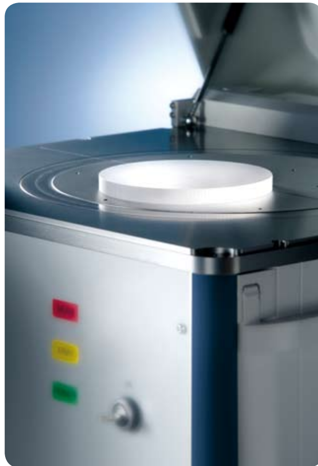
Figure 1. D2 CRYSO close-up showing open lid and crystal in measurement position.
